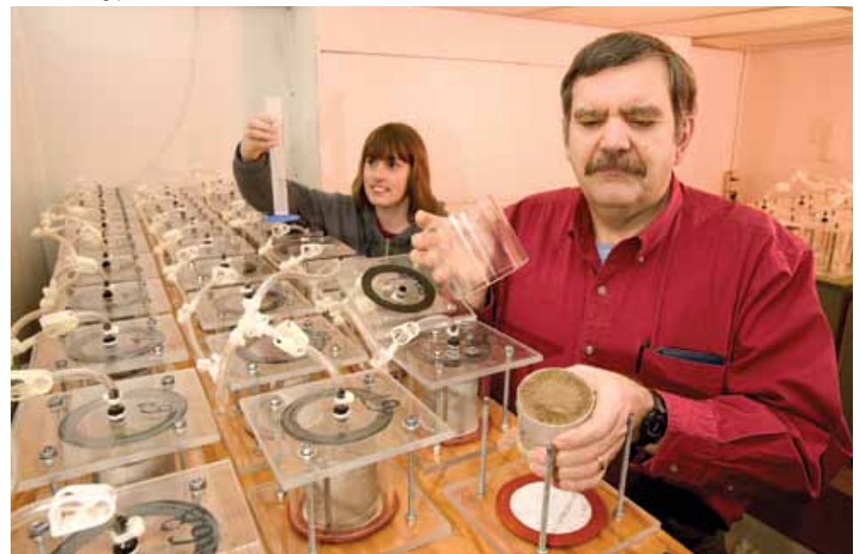
Soil scientist Joseph Benjamin and technician Stacey Poland measure water-holding characteristics of soil using pressure cells.
