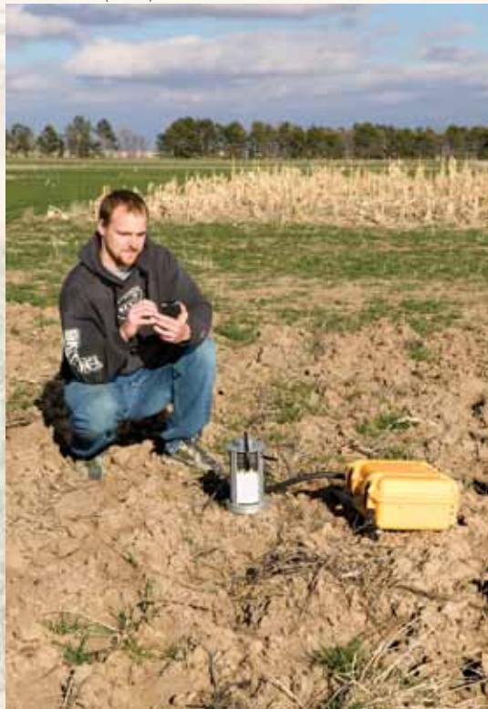
In an alternative cropping system plot, technician Brandon Peterson measures carbon dioxide loss due to tillage.
